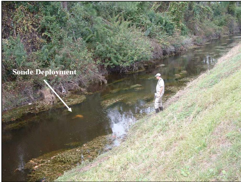
Figure 3. Typical sonde deployment structure and positioning in stream.
